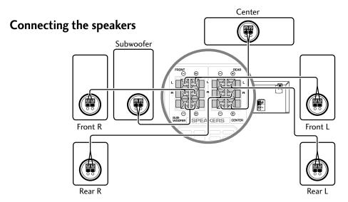
The speaker terminal tabs and supplied speaker cables are color-coded for simpler connection.
